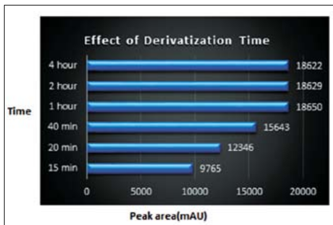
Fig. 2a: Reaction kinetic study with increasing time in acidic condition at 50°C for derivatization
